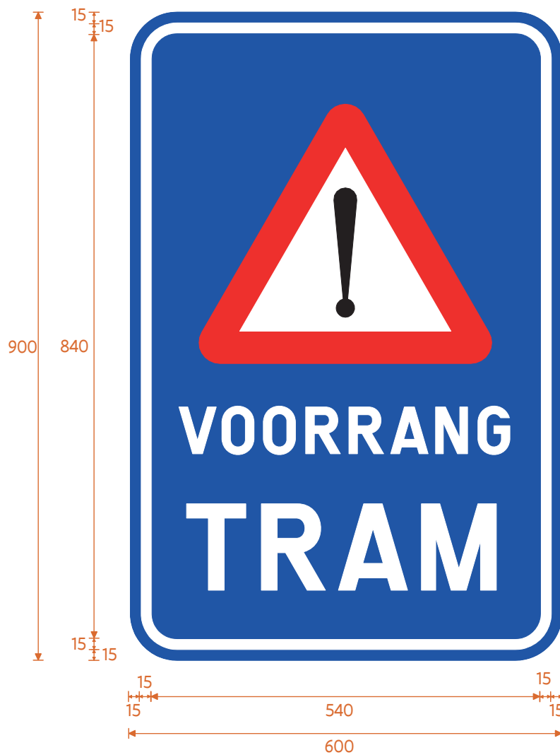
Details bord "voorrang tram" (in mm)
